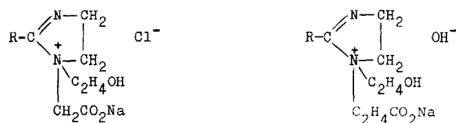
Fig. 1. Conventional structures of imidazoline amphoteric surfactants. Left: derived from sodium chloroacetate; right: derived from ethyl acrylate and/or acrylic acid (salt-free type).
